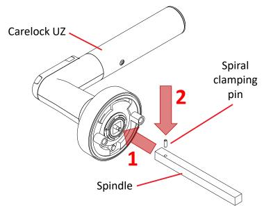
The spindle must be assembled before you can mount Carelock UZ on a door.
