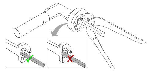
Press the spiral clamping pin all the way in, using adjustable pliers (this is the trickiest part of the installation because of the tiny size of the spiral clamping pin).
